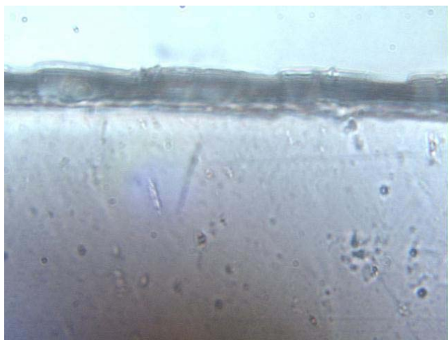
Figure 1. Razor slitting BOPLA film
