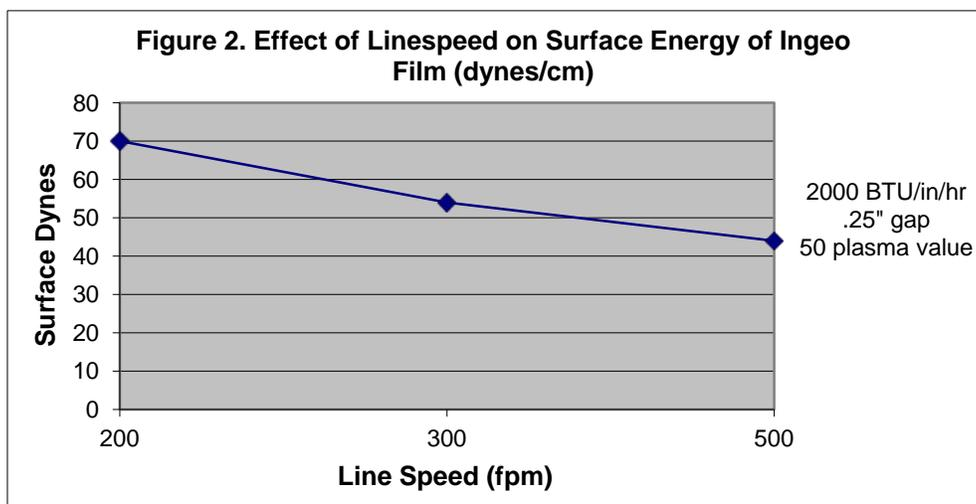
Figure 2 shows that when the line speed increases, the surface energy drops when using a fixed burner output and burner gap. This indicates that the burner output must increase as the line speed increases to maintain a high surface energy and subsequently the burner gap must be increased to prevent the film from distorting from the heat of the flame.
