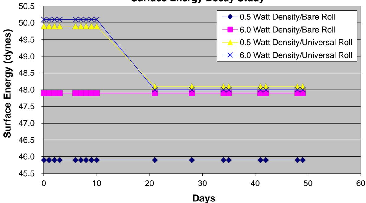
Figure 5 shows untreated Ingeo film does require more watt density to effectively increase the surface energy when compared to "bump" treatment, but not an unreasonable amount of watt density is required to be effective.
