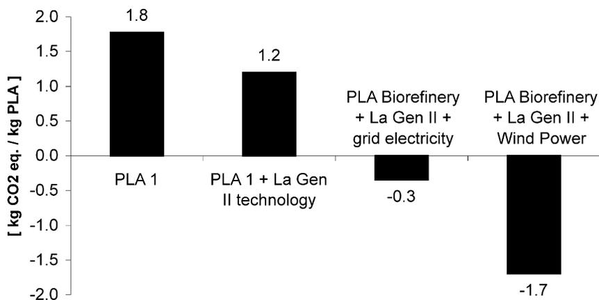
Fig. 12. Potential reduction of greenhouse gasses associated with PLA production.
