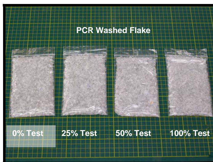
Figure 4 – PCR Flake Samples used for Plaque Let-Down Study (left to right – 0, 25, 50, and 100% Test Flake Blends)
